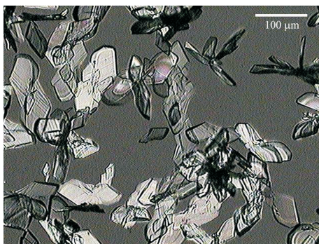
Fig. 5 Optical micrographs of undissolved AFR-PEPA-4 oligomer crystals in NMP at room temperature
